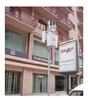
The ETL 2000 provides quality data utilising a central station software @COM3000 remotely retrieving data via landline modem or GSM, either from a single ETL or a network of units.
