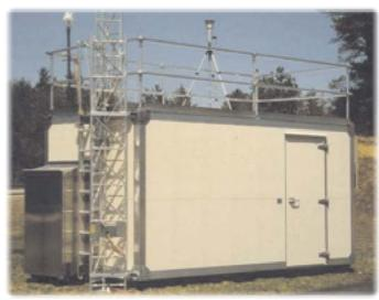
Doors are made of the same construction as the shelter, fully gasketed to obtain an air and rain tight enclosure. The supplied skids and lift/tie down rings facilitate handling by forklift, crane, and rotary or winged aircrafts. Shelters are designed and structurally analyzed by structural engineers to meet the applicable requirements of numerous codes, such as UBC, SBCC, etc. Electrical installation conforms to the latest issue of the NEC, CSA, IEC or other applicable foreign codes.
